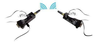
Parani-SD1000 provides Pairing Button for instant configuration without a PC to make an automatic connection between two Parani-SD1000s. (Refer to the two Parani-SD1000s as SD1 and SD2, respectively)
