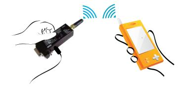
Using pairing button, users can make a pairing connection between a Parani-SD1000 and other Bluetooth devices. (Refer to the Parani-SD1000 as SD1)
