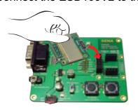
3 Connect the serial cable to the Development Board
