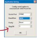
Parani-ESD Series default configuration is 9600 bps Baud rate, 8 Data bits, No. Parity, 1 Stop bit and H/W flow control
